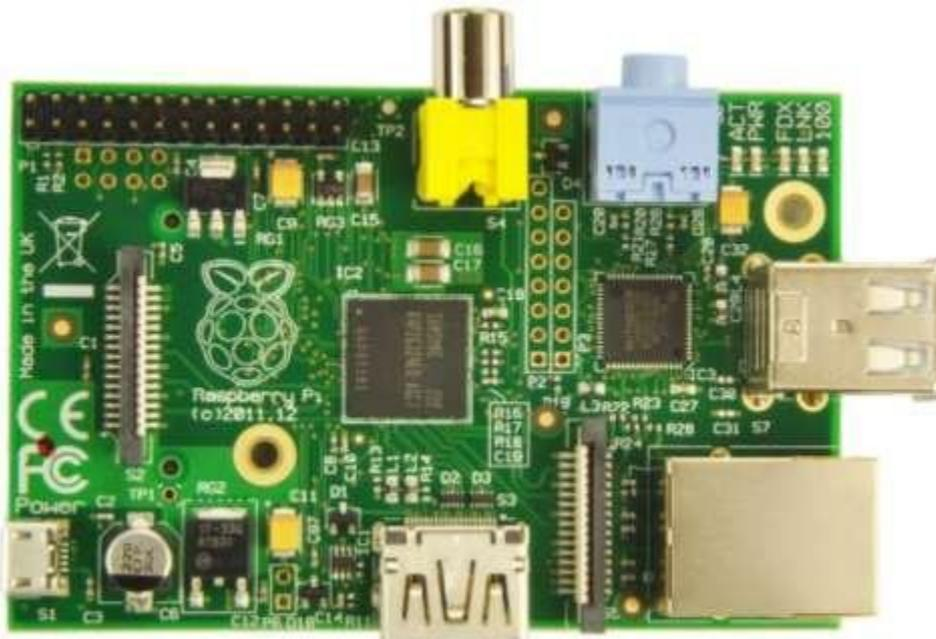
Figura 1, Circuito embarcado RaspberryPi Rev. 2.
